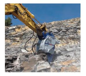
In even 70% of the job applications a 2 to 5 times higher production can be achieved. The Xcentric® Ripper's closed energy chamber cannot be influenced or damaged from the outside by dust, water, dirt or what so ever. This means that it can work without any problem in the most severe conditions in tunnels, foundations, muddy and wet places.
